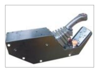
7. It is recommended that the controls are mounted in-place of the seat armrest on the side of the cutting head. A pivoting bracket is supplied with every machine, if additional brackets are required contact your local dealer. A 12v/30Amp power supply will be required.
