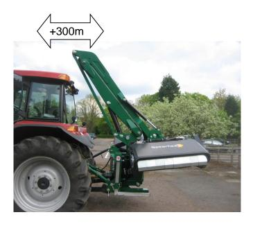
4. Carefully position main boom over the tractor cab roof until rubber bump stop meets the flip-over transport bracket, allow minimum of 300mm.
