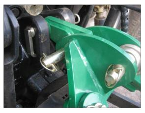
2. Fit stabiliser bracket into top link clevis and fit top link. The standard link comes with a Cat III hole plus a Cat III to Cat II reducing bush, a 28mm bracket is available on request.
