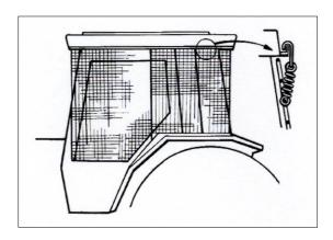
10. Use only tractors with safety glass. If windows are not laminated safety glass, polycarbonate glazing must be fitted between operator and cab meshing. Shape mesh to cover all windows that the driver will look through to view flail head in any operating position. Mesh can be retained by springs and clips supplied, but it is the operator's responsibility to ensure guarding is firmly in place.
