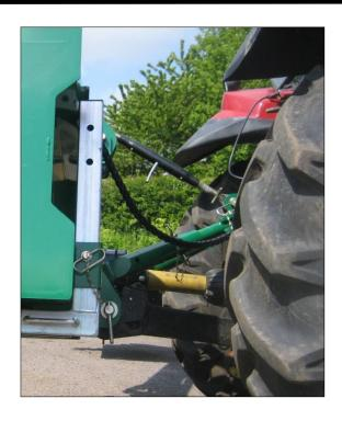
4. Raise machine to required height. Both P.T.O. shafts should be roughly in-line, an upward angle of up to 17° is acceptable to ensure adequate clearance.
