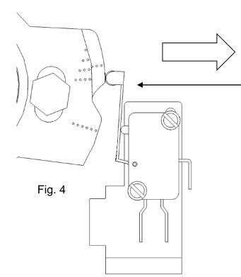
Ensure the switch lever closes the contacts, if not adjust by bending the lever arm towards the cam.
