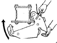
3. Fit lift-in hitch assembly
