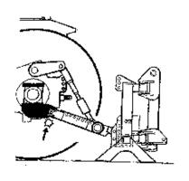
7. Ensure top link is fitted to prevent machine from tipping over before raising. Lift sub frame until it engages in the catches. Note: It is best to mount the sub frame to the tractor first.
