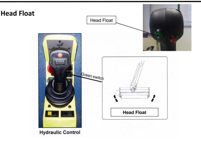
This option allows the flail head to follow contours of the ground without having to constantly control the angle of the head.
