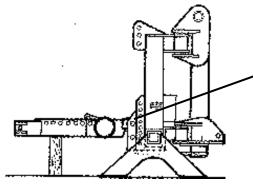
4. Assemble sub frame to suit axle width 1m or 1.1m, mount sub frame assembly to your machine using bottom pin holes.
