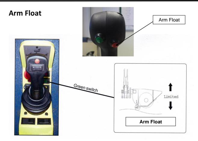
This is only to be used in verge mowing set up, it will reduce weight on the rear roller allowing head to move more easily, following small changes in ground contours in a forward motion, with the aid of a pre-charged gas accumulator.
