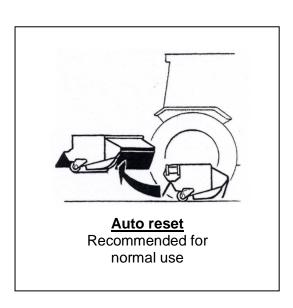
Never attempt to operate the machine when travelling backwards, the break back will not function and any damage caused will not be considered warranty. The break back feature does not excuse the machine operator of their need to be aware of obstacles and to avoid hazards. It is your responsibility to maintain a long reliable working life.
