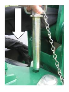
6. Fit slew locking pin to secure slew post to A frame.
