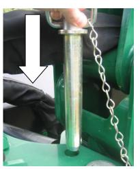
5. Fit slew locking pin to secure slew post to A frame.
