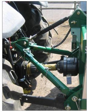
3. Fit stabiliser tubes between A frame and stabiliser bracket. Ensure the tubes are free to slide, do fit locking pins.
