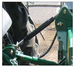
5. Adjust the top link so that the machine sits vertically.
