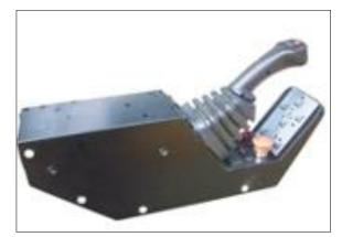
7. It is recommended that the controls are mounted in-place of the seat armrest on the side of the cutting head. A pivoting bracket is supplied with every machine, if additional brackets are required contact your local dealer. A 12v/30Amp power supply will be required.
