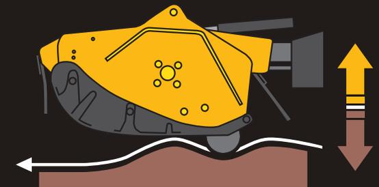
ROBOCUT T600 & T800 are both fitted with a fully programmable hydraulic attachment floatation system that ensures optimum performance in all conditions.
