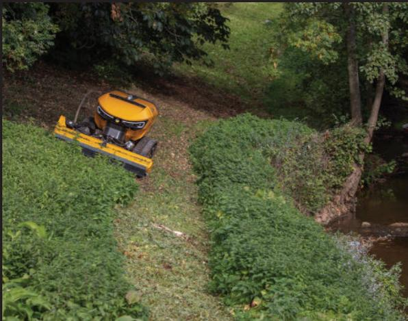
All McConel ROBOCUT's are fitted with engine technology which have been developed in partnership with OEM manufacturers specifically for working on steep gradients of 55 degrees whilst meet latest emission legislation.
