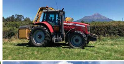
TWO OF THE COMPANY'S MASSEY FERGUSON TRACTORS HAVE DYNAVT CONTINUOUSLY VARIABLE TRANSMISSIONS, WHICH MAKE THEM VERY GOOD FOR HEDGE TRIMMING.
